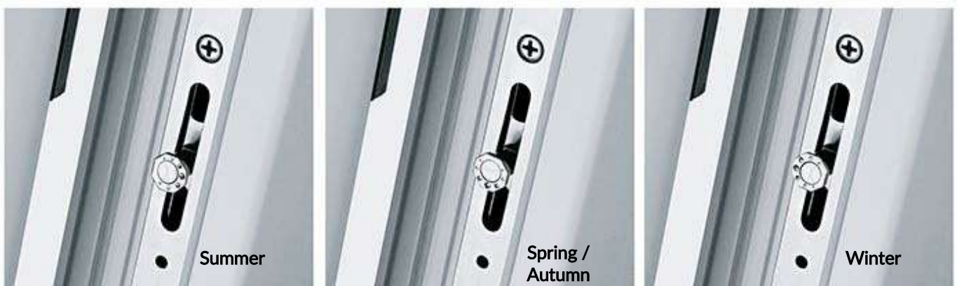
Setting of the activPilot cam bolt for summer and winter
