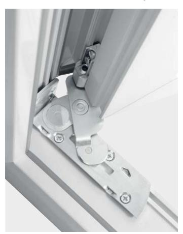
With just two add-on components – a sash hinge rail and adapter plate – you can increase the load bearing capacity from 100 kg to up to 150 kg.
